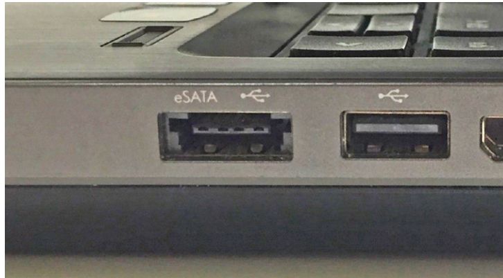
FIGURE 2.46 USB over eSATA
