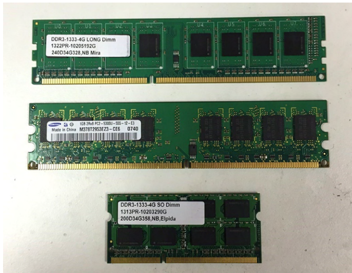
FIGURE 1.19 Memory module form factors
