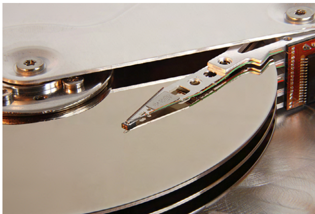
FIGURE 1.20 Inside a hard drive
